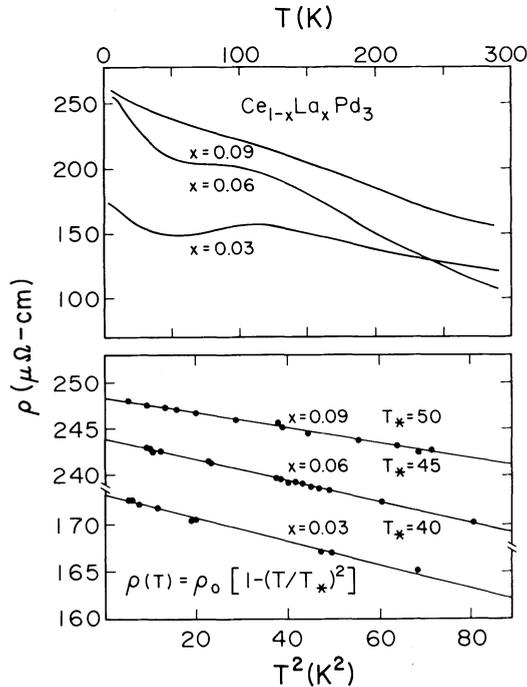
Fig. 5. (Top) Resistivity of  $\text{Ce}_{1-x}\text{La}_x\text{Pd}_3$  for  $x = 0.03$ ,  $0.06$  and  $0.09$ ; (bottom) Low temperature resistivity plotted vs.  $T^2$ . Values of  $T_*$  are given in the figure.
