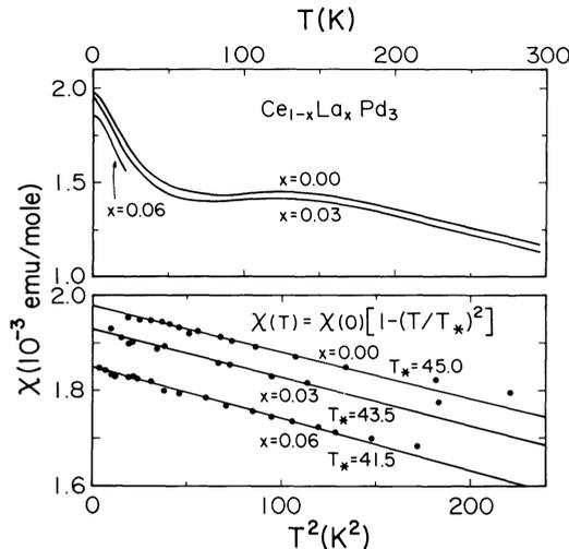
Fig. 6. (Top) The susceptibility of Ce<sub>1-x</sub>La<sub>x</sub>Pd<sub>3</sub> vs. temperature for  $x = 0, 0.03$  and  $0.06$ ; (bottom) The low temperature susceptibility plotted versus  $T^2$ . The power law is  $\chi(T) = \chi_0(0)[1-(T/T_*)^2]$ , with  $T_*$  given in the plot.
