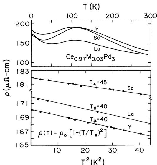
Fig. 4. (Top) The resistivity of Ce<sub>1-x</sub>M<sub>x</sub>Pd<sub>3</sub> plotted versus temperature for  $M = Y, Sc, La$ ; (bottom) The low temperature resistivity of the same three compounds plotted vs.  $T^2$ . These demonstrate the power law behavior  $\rho(T) = \rho_0 [1 - (T/T_*)^2]$  with  $T_*$  given in the plot.
