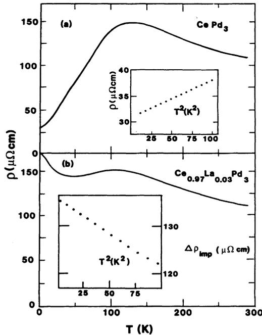
Fig. 1. Resistivity at ambient pressure for (a)  $\text{CePd}_3$  and (b)  $\text{Ce}_{0.97}\text{La}_{0.03}\text{Pd}_3$ . This inset in (a) shows the low temperature resistivity of  $\text{CePd}_3$  plotted vs.  $T^2$ . The inset in (b) shows the impurity contribution (i.e., with the resistivity of  $\text{CePd}_3$  subtracted out) to the resistivity of  $\text{Ce}_{0.97}\text{La}_{0.03}\text{Pd}_3$  plotted vs.  $T^2$ . (From Ref. 5)
