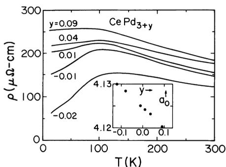
Fig. 2. Resistivity of  $\text{CePd}_{3+y}$  for several values of  $y$ . The inset shows the lattice constants as a function of  $y$ .
