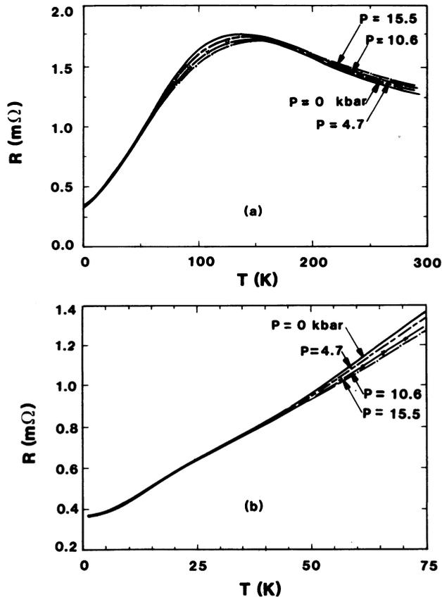
Fig. 3. (a) The resistance of  $CePd_3$  versus temperature for four pressures; (b) Low temperature region of the data for the same four pressures showing the insensitivity to pressure below 40K. (From Ref. 5)
